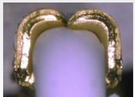
Covered crimping core wire
