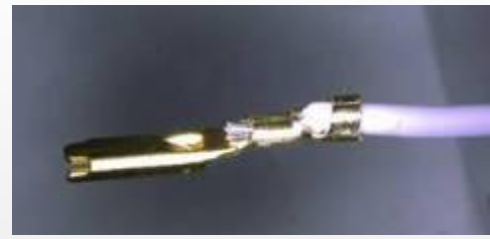
Contact pin crimping
